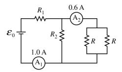
9. The figure above shows a circuit containing four resistors, a battery, and two ammeters. The current in ammeter A<sub>1</sub> is 1.0 A, and the current in ammeter A<sub>2</sub> is 0.6 A. The two resistors labeled R are identical. What are the currents in R<sub>2</sub> and in each of the two resistors labeled R?
